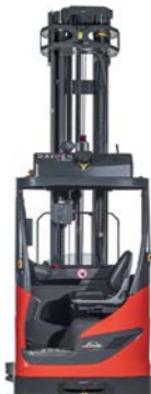
R-Matic 1.6 Ton Automatic / Manual Driving Geoguidance Navigation
