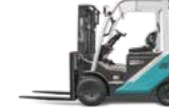
Dedicated Li-Ion Battery ECB Forklift
